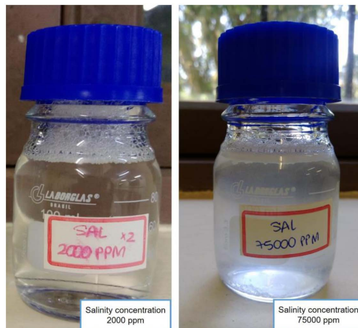
Figure 4—Images showing examples of the aqueous stability test results at salinities of 2000 and 75000 ppm at fixed concentrations of the surfactants (1000 ppm) DEA (1.5 mM) and PSM (100 ppm).
